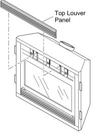
Figure 42 - Removing Top Louver Panel
